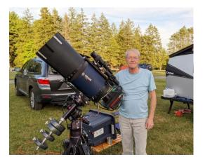
My usual EAA setup consists of an 8" Celestron SCT optical tube @ f6.3 with a ZWO ASI294MC Pro camera and filter wheel on an Atlas EQ GEM mount, along with a piggybacked Canon CCTV 25-100mm zoom lens with ASI290MC camera, and a 60mm Antaries refractor guidescope with an ASI120MC camera. I also setup my DIY Allsky cam, a ZWO ASI224MC & fisheye lens inside a domed container on a tripod mount.
