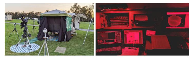
I also setup the Allsky cam (ZWO ASI224MC & fisheye lens in a DIY dome), and my 'Guttercam' (Samsung SDC435 analog security camera & widefield lens in a drain-gutter enclosure) that I use to monitor the main telescope as it slews. Setting Guttercam up to the south of the telescope also allowed it to do double-duty to monitor for aurora.
