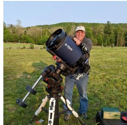
After getting camp squared away, I assembled my telescope: a 8" Celestron SCT optical tube @ f6.3 with a ZWO ASI294MC Pro camera, filter wheel and focuser on an Atlas EQ GEM mount, along with a piggybacked Sky-Watcher EVO 50mm refractor with ASI290MC camera, and a 60mm Antaries refractor guidescope with an ASI120MC camera. I also setup the Allsky cam, a ZWO ASI224MC & fisheye lens in a DIY dome. A little later, I setup the blackout tent off the back of the camper's clamshell.
